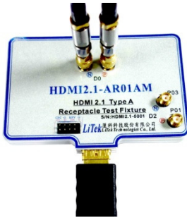
Fig 2: HDMI2.1-AR01AM plugged into Host Device after Type A to Type A cable assembly
